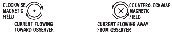
(C) Direction of current flow through conductors determines direction of magnetic field around conductors.
